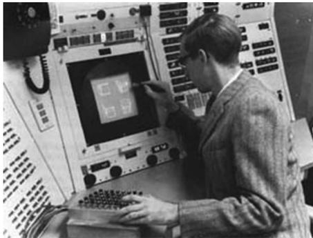
**Fig. 1.5** The use of the sketchpad software with a light pen to create precise drawings
