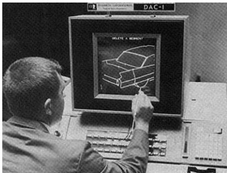
**Fig. 1.6** The first CAD system by IBM (called DAC-1)—DAC stands for *Design Augmented by Computer*
