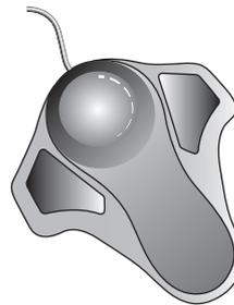
Fig. 10.5 Trackball device
